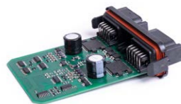
Control for a retractable landing gear
