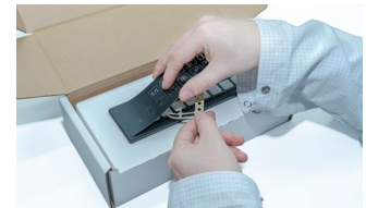
Applying the customized operating foil
